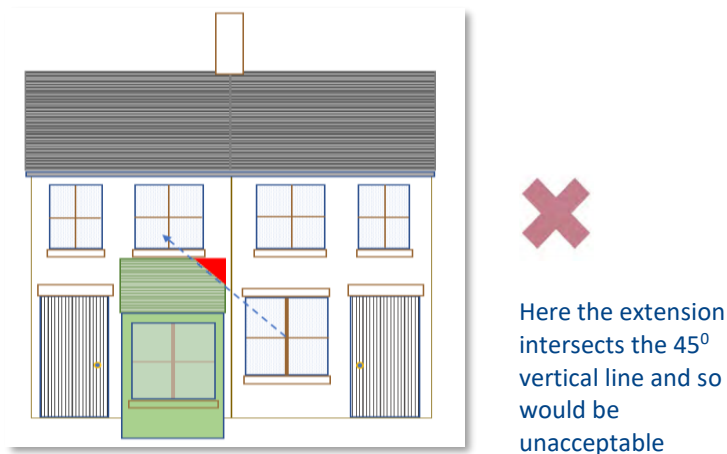
Figure 10: The 45° Rule diagram – front view
